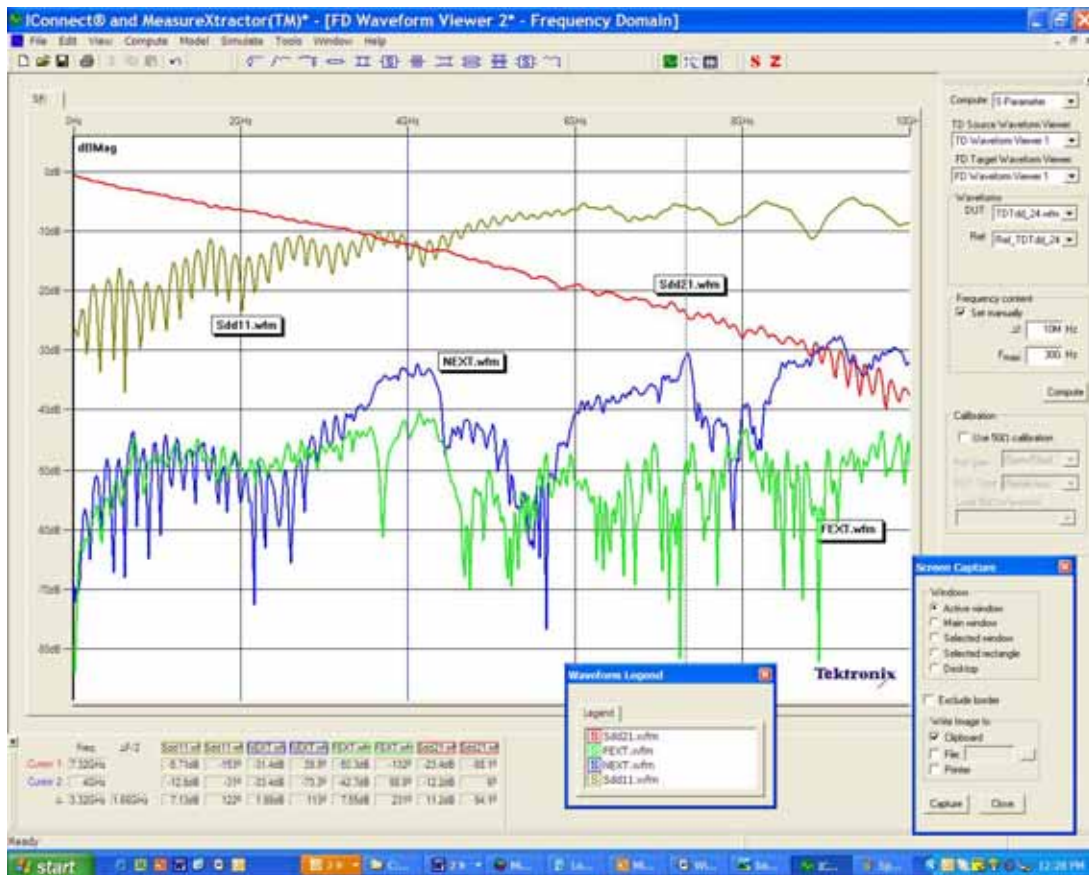
Figure 4. S11 is the reflectivity of a signal injected from the left and S12 is the transmissivity of that signal; S22 is the reflectivity of a signal injected from the right and S21 is the transmissivity of that signal. The situation is more complicated in differential systems – a complete set of S-parameters for differential and common-mode stimulus and response result in a total of 16 parameters – but the idea is the same.
