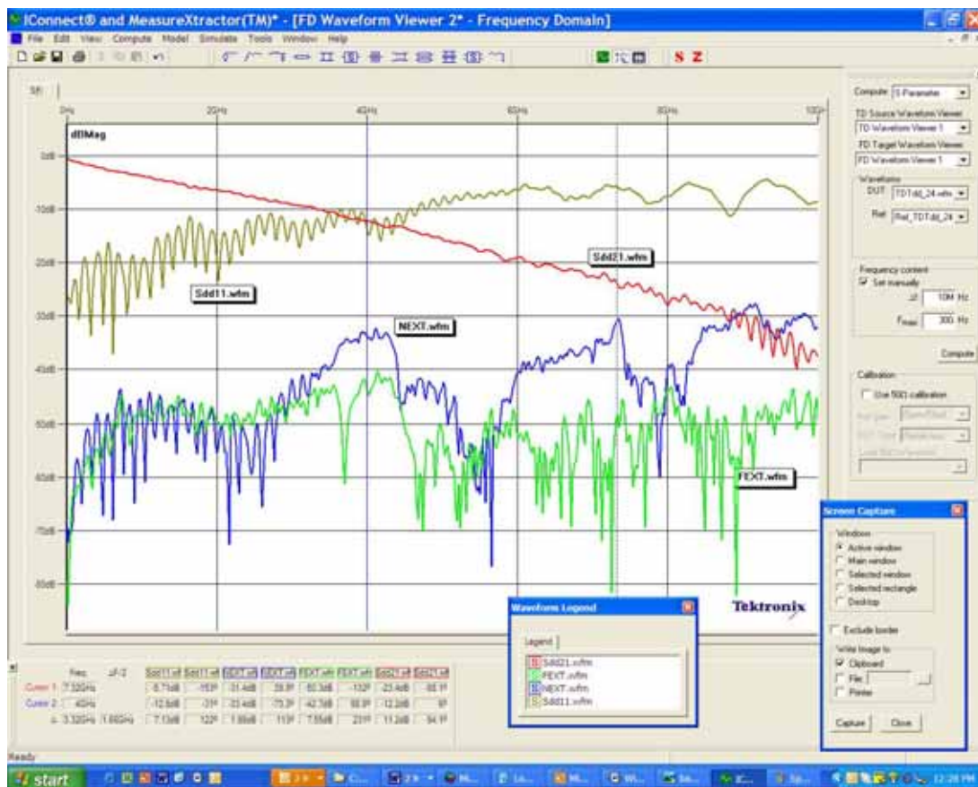
Figure 4: S-parameters measure the frequency response of transmission and reflections from both ends of a device.
